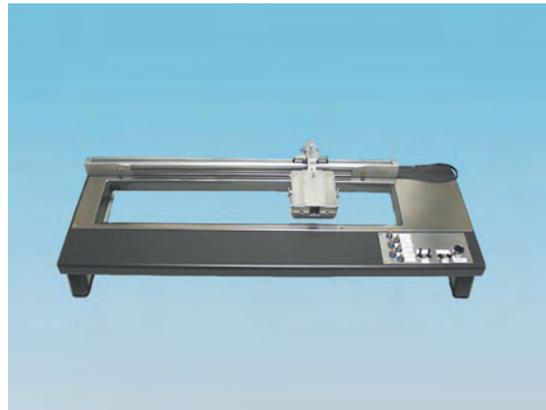
**Abb. 9** Labuda Linear-Wischsimulator Mark II
